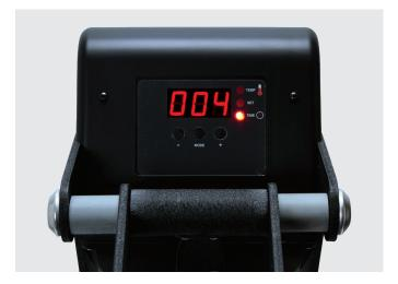
Once you have adjusted the temperature, press the Mode Select button again to advance to Time Mode.
