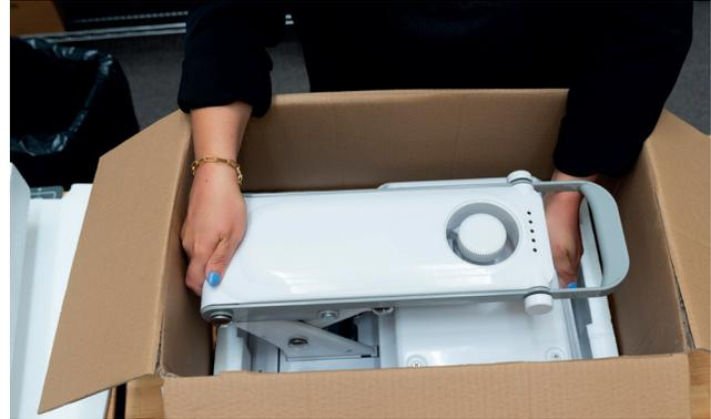
Place the press in the box carefully, ensuring that the press sits on the bottom foam completely.
