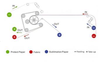
full-automation, quality electric parts and components, like all other Easty machines. The Calender has an oil filled drum that ensures consistent heating throughout the drum surface. Its dual layer hard chrome drum diameter is 8.27" (210mm), which can operate at 230°C of temperature, achieving high transfer speed with strictly even temperature. Both air expansion shaft and conveyor belt can be upgraded for more user-friendly operation as well.
